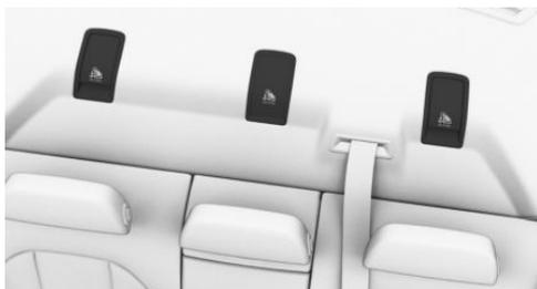
Depending on the features installed in the vehicle, there are two outer mounting points or three other mounting points for child restraints with tether straps.
