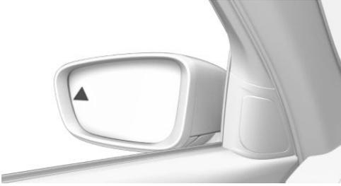
The light in the exterior mirror flashes if other vehicles are detected by the rear sensors when the vehicle is reversing.
