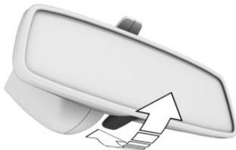
To reduce glare tilt the lever on the rear-view mirror forward.
