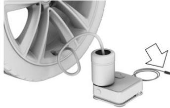
6. Switch on the compressor with standby state switched on or the engine running.
