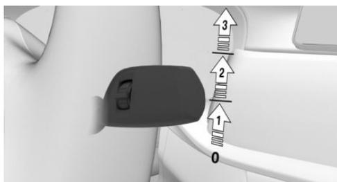
Press the lever upwards once from the home position, arrow 1.
