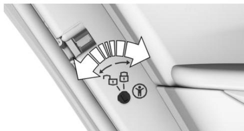
Unlock or lock the safety switches on the rear doors with the integrated key.
