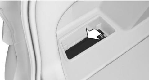
The on-board tool kit is located in the left storage compartment of the boot, under a cover.
