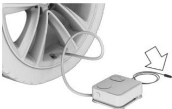
5. Switch on the compressor with standby state switched on or the engine running.
