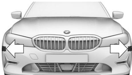
Depending on the equipment, there are two additional radar sensors in the front bumper.
