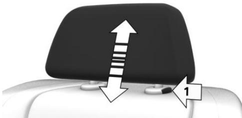
The outer head restraints can be adjusted in height.
