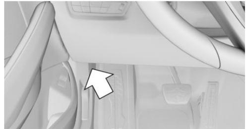
The OBD socket for checking emissions-relevant components is located on the driver's side.
