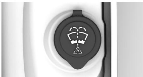
The reservoir for the washer fluid is located in the engine compartment.
