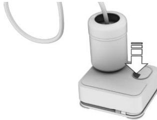
Let the compressor run for approximately 10 minutes to fill the sealing compound and achieve a tyre inflation pressure of approximately 2.0 bar.
