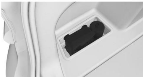
The Mobility System is located in a bag in the left storage compartment of the boot. To remove it, loosen the tensioning strap.
