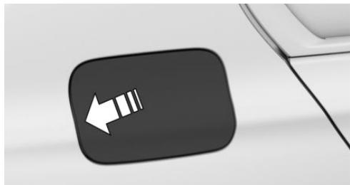
2. Turn the fuel tank cap anticlockwise.
